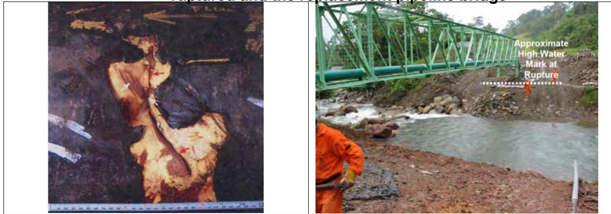
Figure 5. Photographs of the open-cut buried pipe section that ruptured and the replacement pipeline bridge 18
